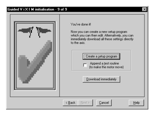
Checking the 'Append a test routine' box will include a simple routine that turns the motor shaft to verify drive operation. To alter any configuration set-up step backwards using the 'Back' button.
